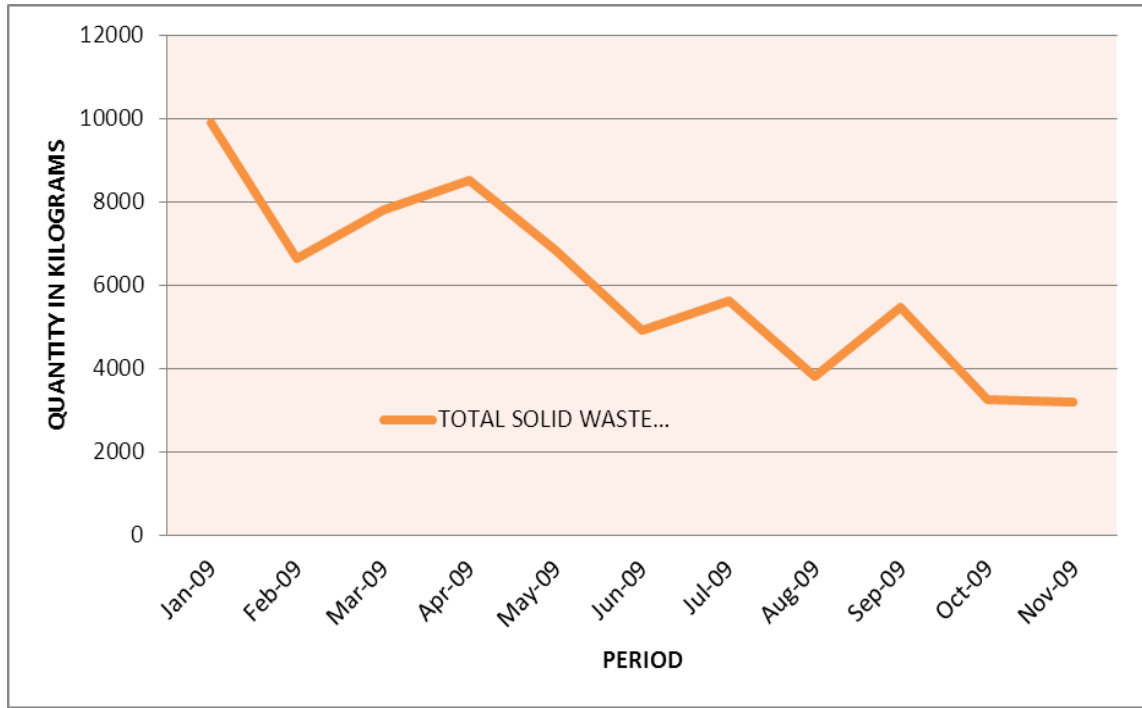
Figure 22 Offsite waste treatment volume trend before (Jan-May) and after (June- Nov) implementation of the source waste reduction measures
