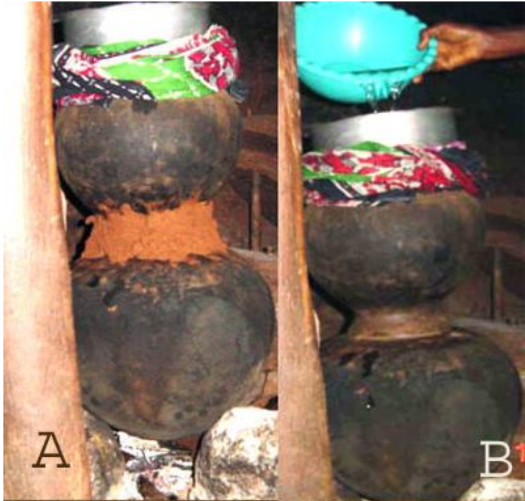
Figure 2.6. Distillation equipment sets (pots). A- a unit with the largest pot having a wide mouth; sealing between the perforated pot and largest pot is enhanced by mud from red soil. B-no mud was applied between the perforated pot and the largest pot
