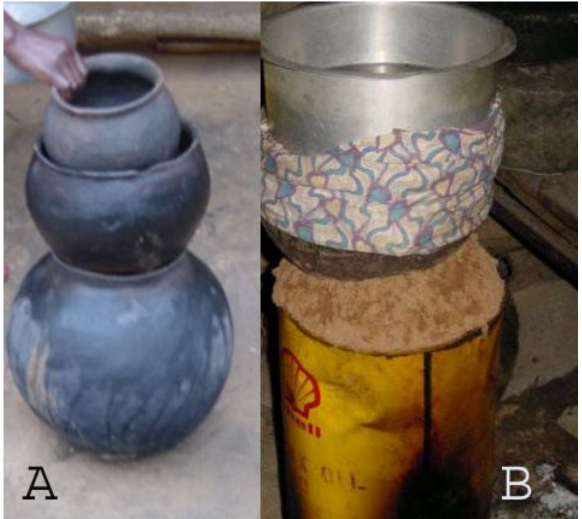
Figure 2.5. Two distillation equipment sets arranged vertically. A-largest pot act as a distiller (reservoir), B- metallic container ( debe ) is used in place of the largest pot.
