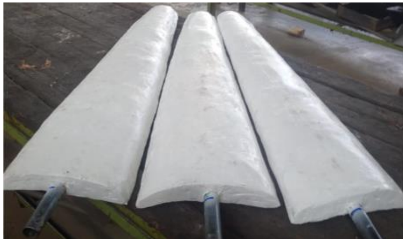
Plate 3.6: Styrofoam Blades Strengthened with Fiber Material
