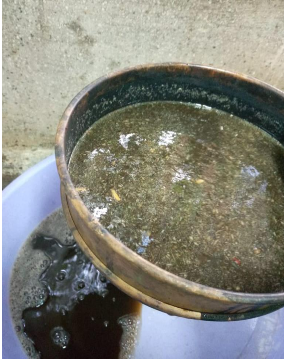
9. Separating solids from liquid by sieving
