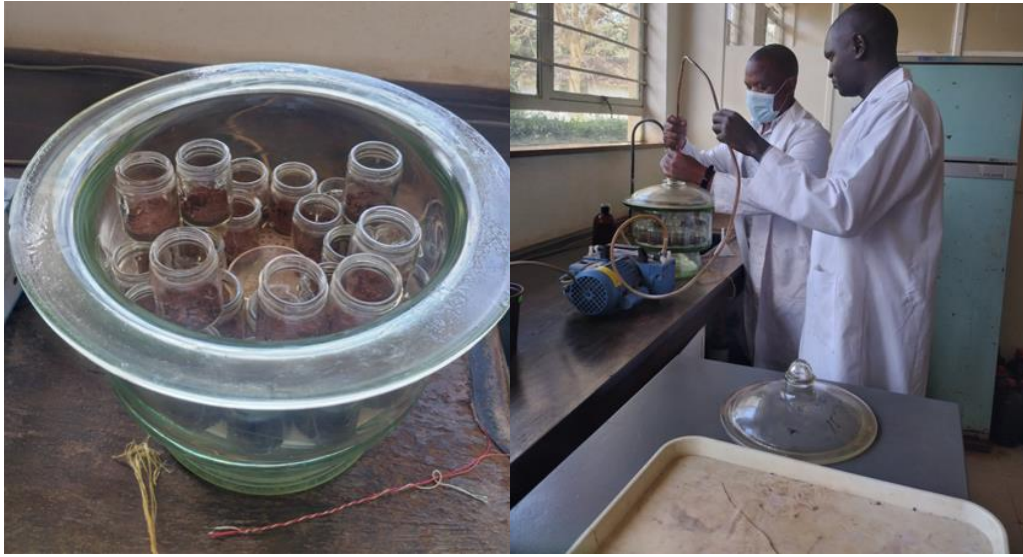
Plate 3.2: Soil Samples Placed in Desiccators for Incubation and Extraction
