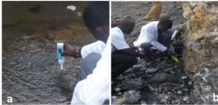
Figure 3.7: Sampling Point Showing Sample Collection and Measuring of Physical Parameters. a) Hot Spring Physical Parameters; b) Offshore of the Lake Soil Sampling.
