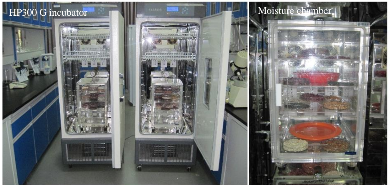
Figure 4.1: Incubators used for storage of seed in a controlled temperature and relative humidity chamber to artificially age the common bean accessions
