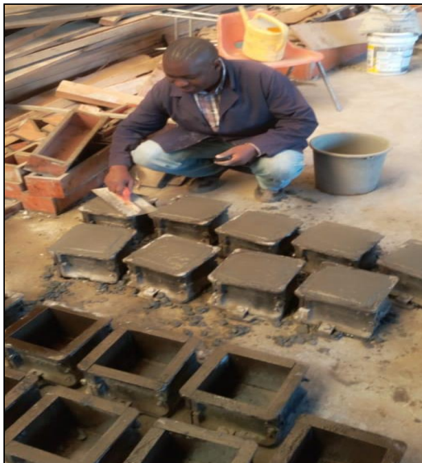
Plate 3.3: Casting cubes for compressive strength test
