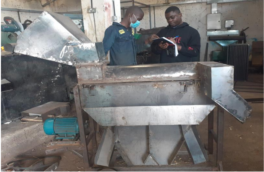
Plate C3: Common bean thresher prototype used for validation
