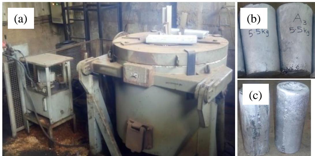
Figure 3.4: Melting of wrought Aluminium scrap: (a) Melting Batch A Scrap Using Oil Fired Furnace; (b) cast Ingots From Batch A; and (c) Billets Cast From Batch C.
