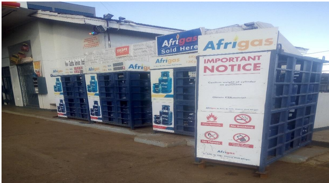
Good practice: Proper cylinder storage and signages
