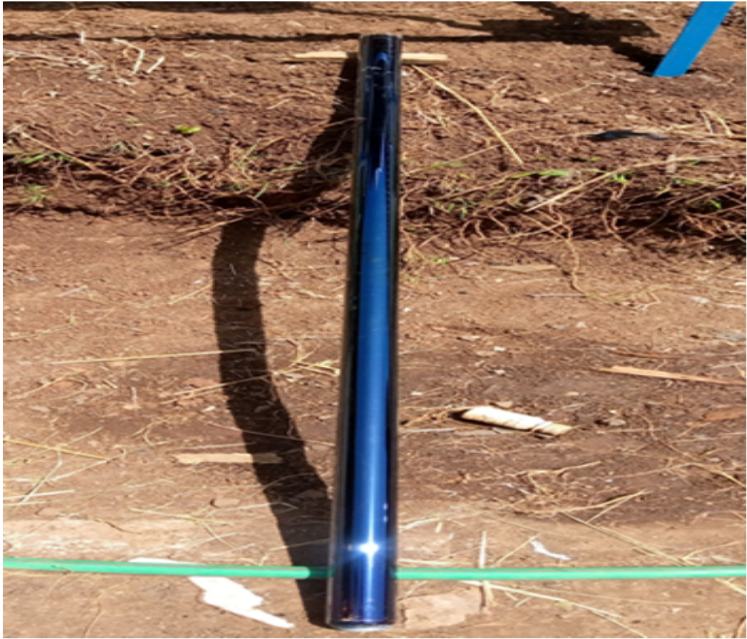
Figure 3.4: Coated Inner Tube Responsible for Solar Absorption
