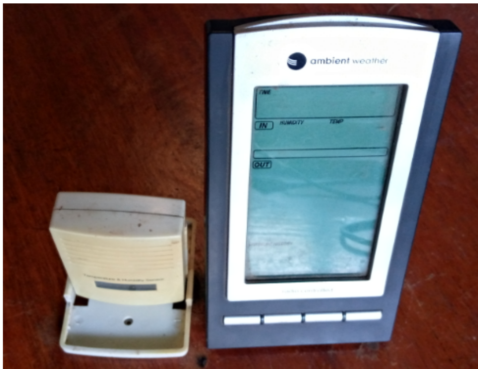
Figure A.2: Weather Station for Measuring Atmospheric Temperature
