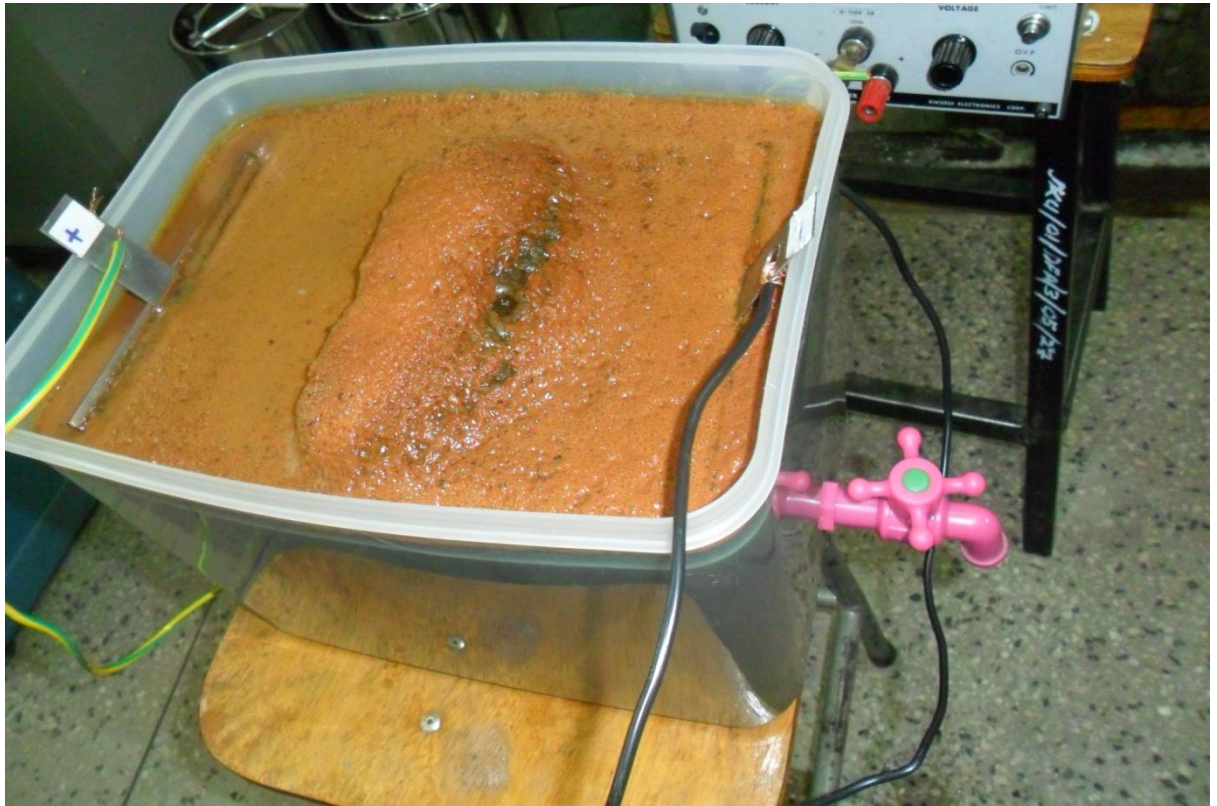
Plate 3: Ongoing Treatment for Iron Plates (with formation of Coagulants)
