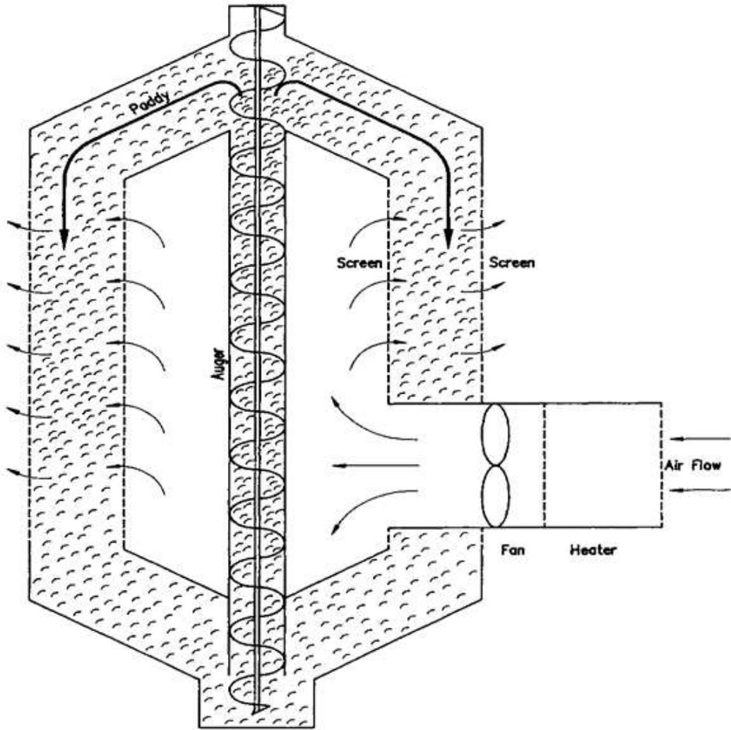
**Figure 2.1: Recirculating Batch Dryer**
