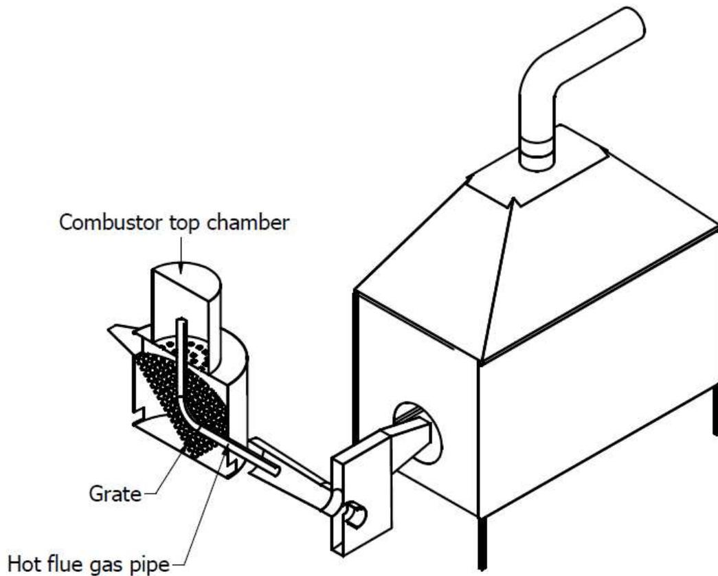
**Figure 3.5 Combustor showing flue gas pipe and grate**
