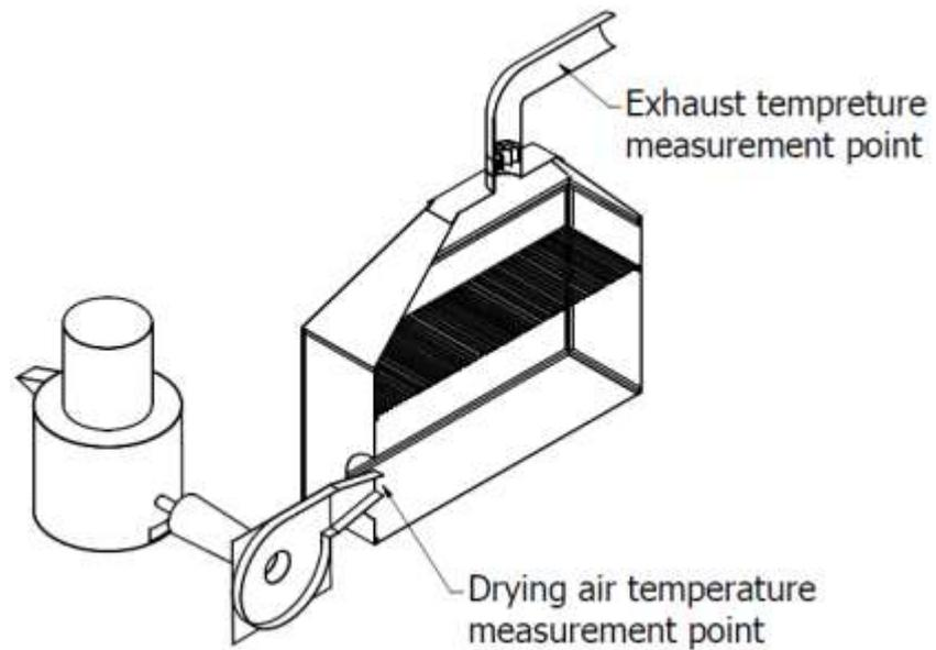
**Figure 3.7: Locations for drying and exhaust temperatures measurements**
