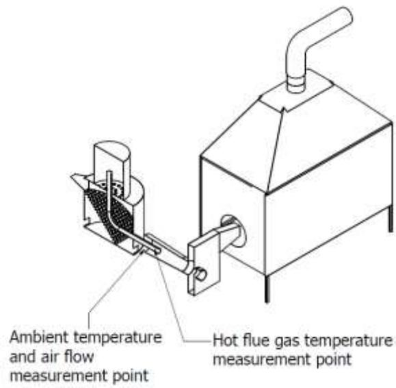
**Figure 3.6: Locations for airflow flue gas and exhaust temperature measurements**
