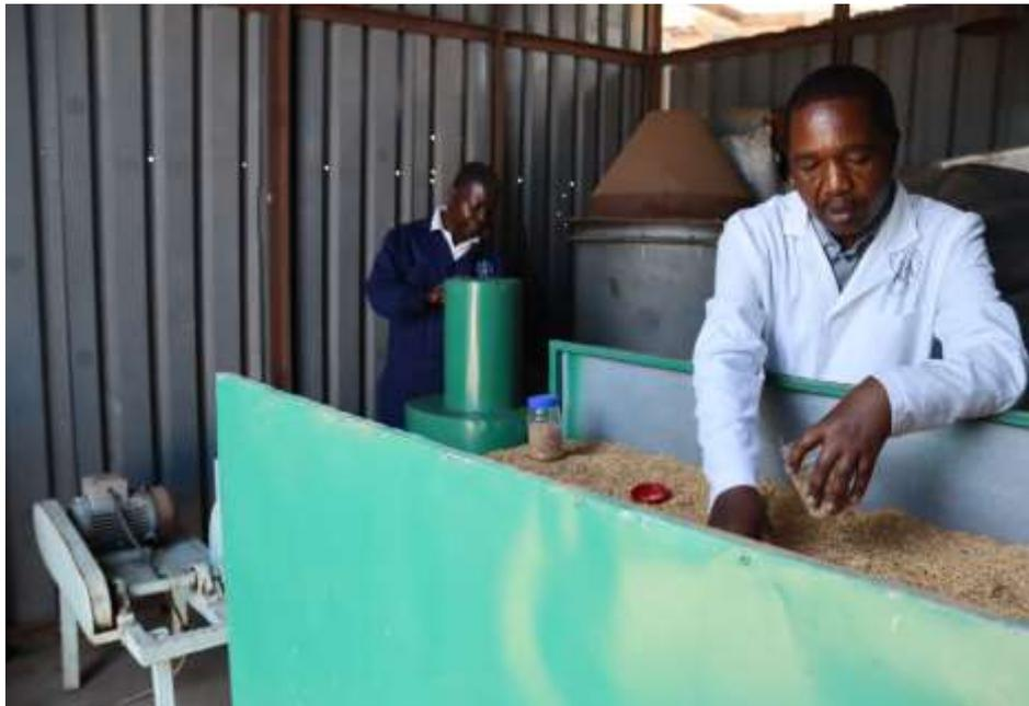
**Figure 3.9: Paddy Drying Bed without an Exhaust Fan**
