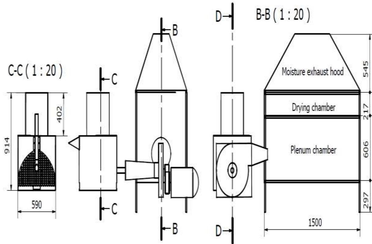
**Figure 3.2: Engineering of Designed Paddy Drying System**
