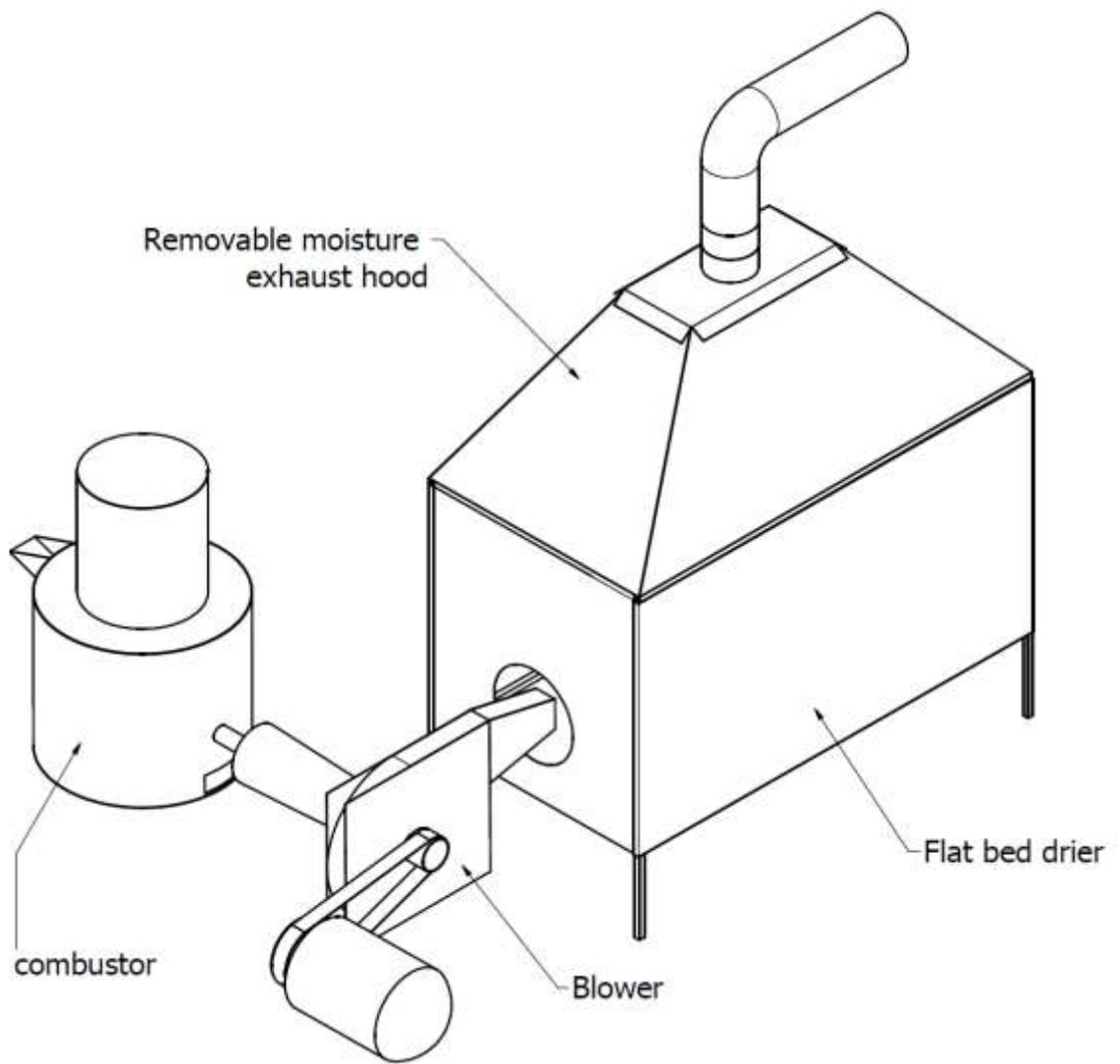
**Figure 3.4 Paddy Drying System with the Exhaust Fan**
