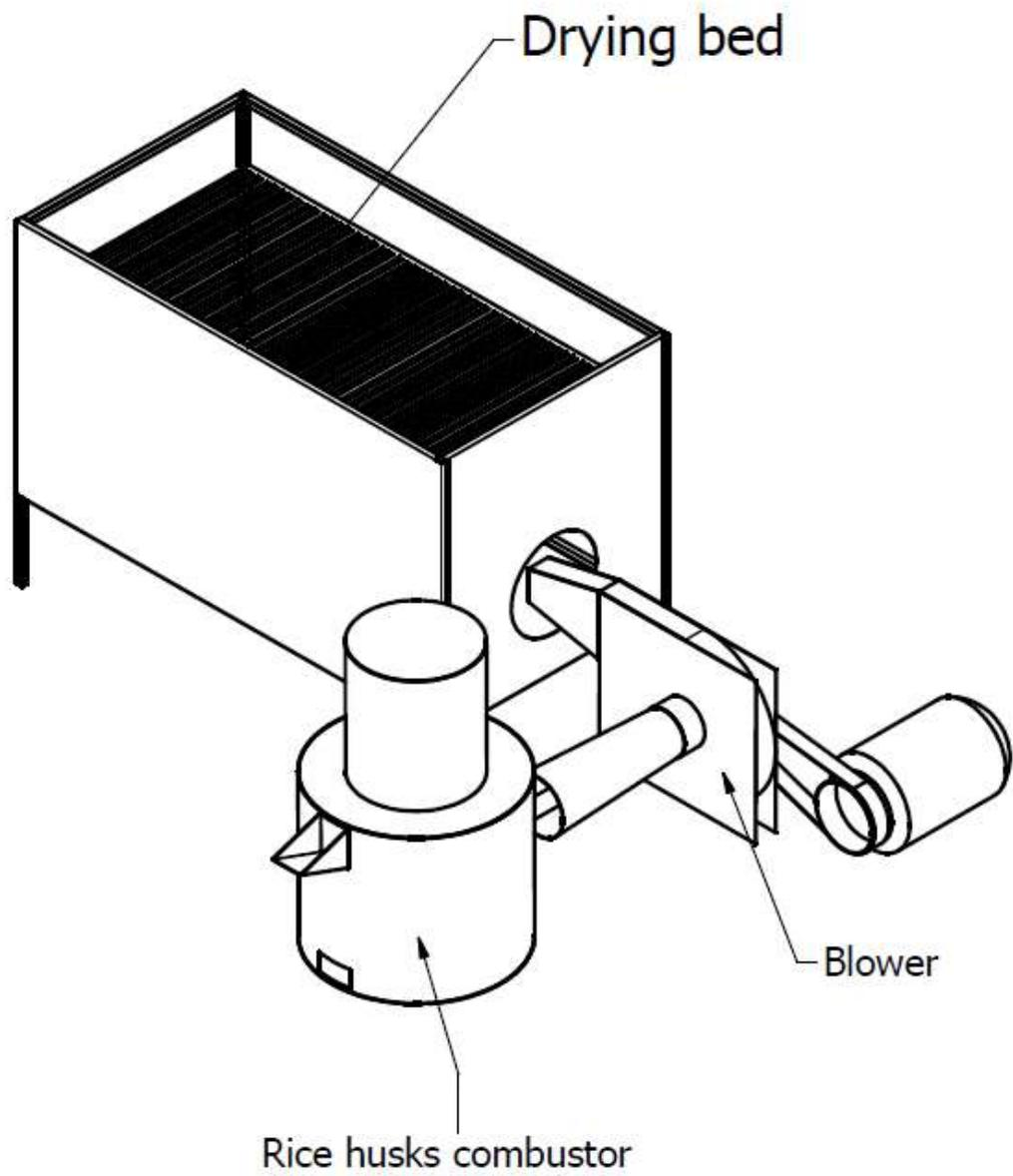
**Figure 3.3 Diagonal View of the Paddy Dryer**
