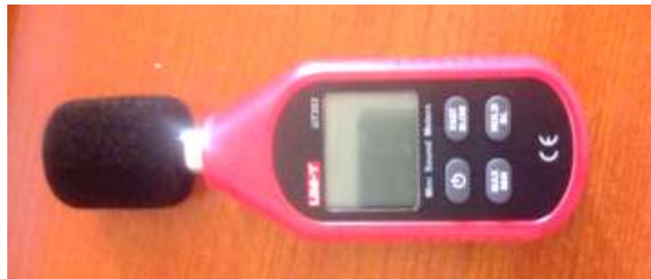
Figure 3.1: A photograph of UNI-T UT353 sound level meter used to measure sound level.
