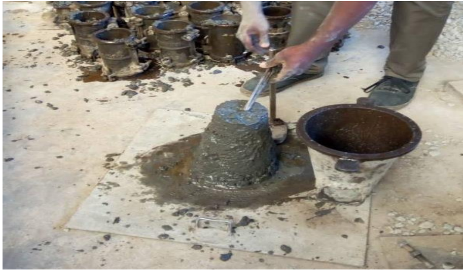
Plate 3: Slump test on the concrete
