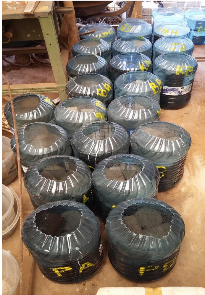
Plate 8: Curing concrete in chemical solution
