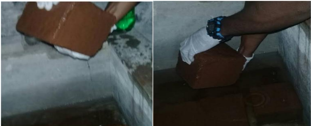
Figure 3.12: Conducting a water absorption test.
