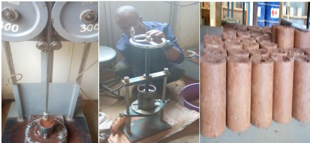
Figure 3.6: Making compressed stabilized cylindrical blocks.
