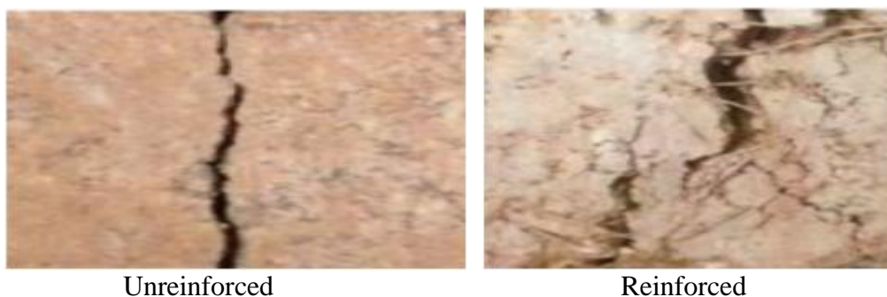
Figure 2.5: Failure of reinforced and unreinforced soil blocks under tension.
