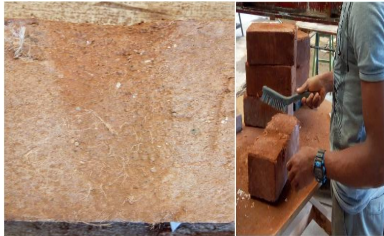
Figure 3.10: Conducting an abrasion test on the blocks.
