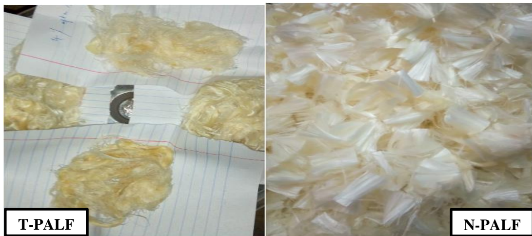
Figure 4.2: Treated and untreated pineapple leaf fibres.
