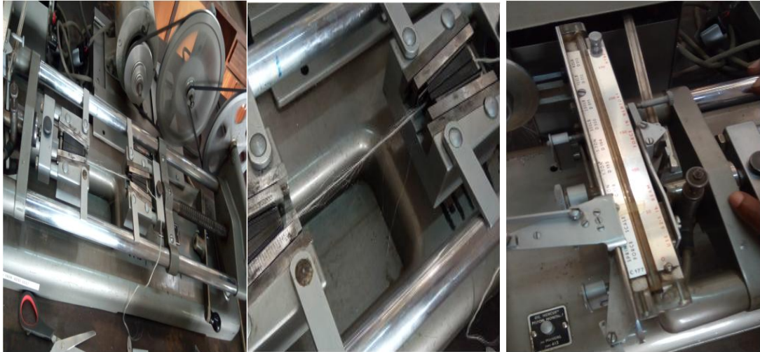
Figure 3.2: Measuring fibre tensile strength using the Hounsfield tensometer.
