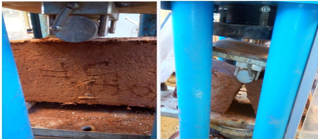
(a) Reinforced (b) Non-reinforced Figure 4.11: Mode of flexural failure for reinforced non-reinforced blocks.
