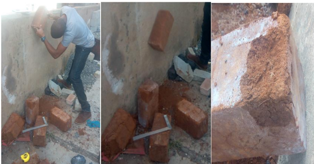
Figure 3.11: Conducting an earth block drop test.
