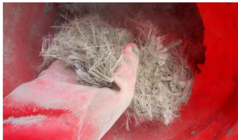
Figure 3.4: Manual mixing of pineapple leaf fibres with cement.
