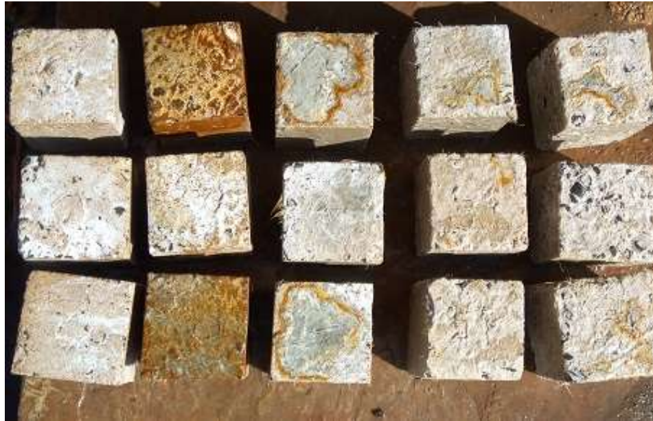
Figure 4- 25: Concrete cubes after 90days of exposure to sulfuric acid solution.
