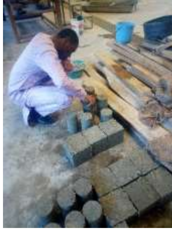
Figure B- 4: Concrete cubes and cylinders specimen for testing
