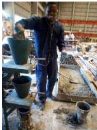
Figure B- 3: Compaction factor measurement
