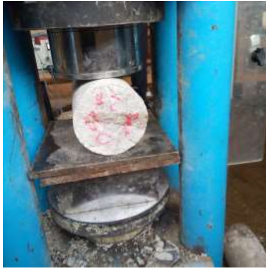
Figure B- 6: Splitting Tensile Testing using UTM Machine
