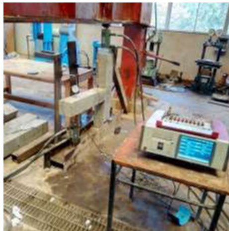
Figure B- 6: Splitting Tensile Testing using UTM Machine
