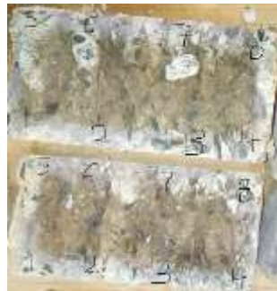
Figure 4- 19: Measuring chloride penetration depth
