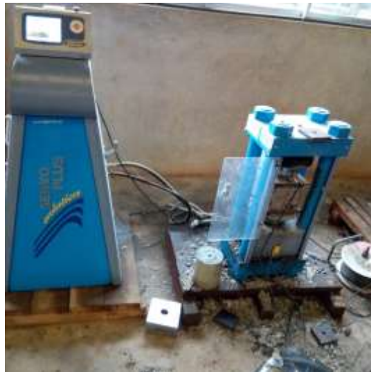
Figure B- 5: Compressive Testing using the UTM machine.
