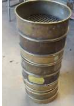
Figure B- 1: BS Test sieves used for Particle size distribution of aggregates.
