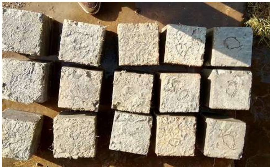
Figure 4- 27: Concrete cubes after 90days of exposure to basic solution.
