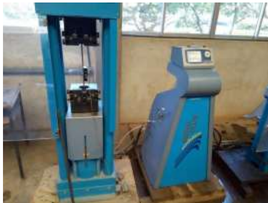
Figure B- 7: Testing of beam-column joints set up
