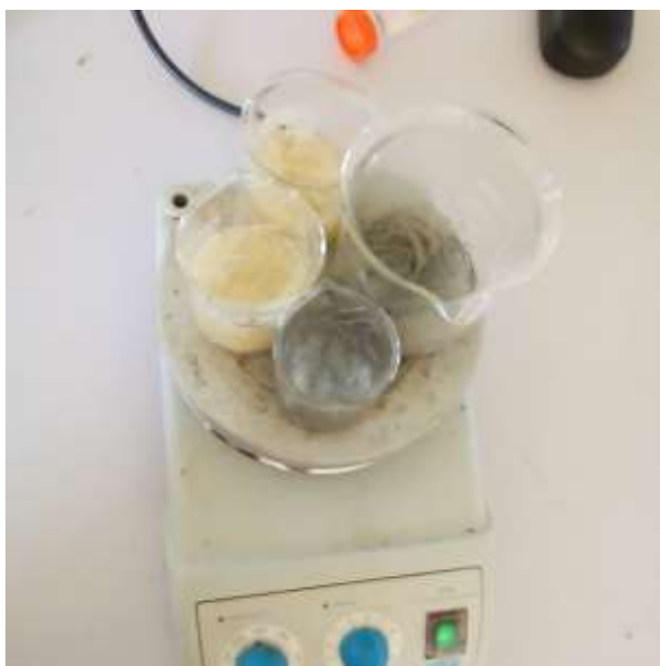
Figure B- 9: Heating of fibers in ethanol for chemical analysis
