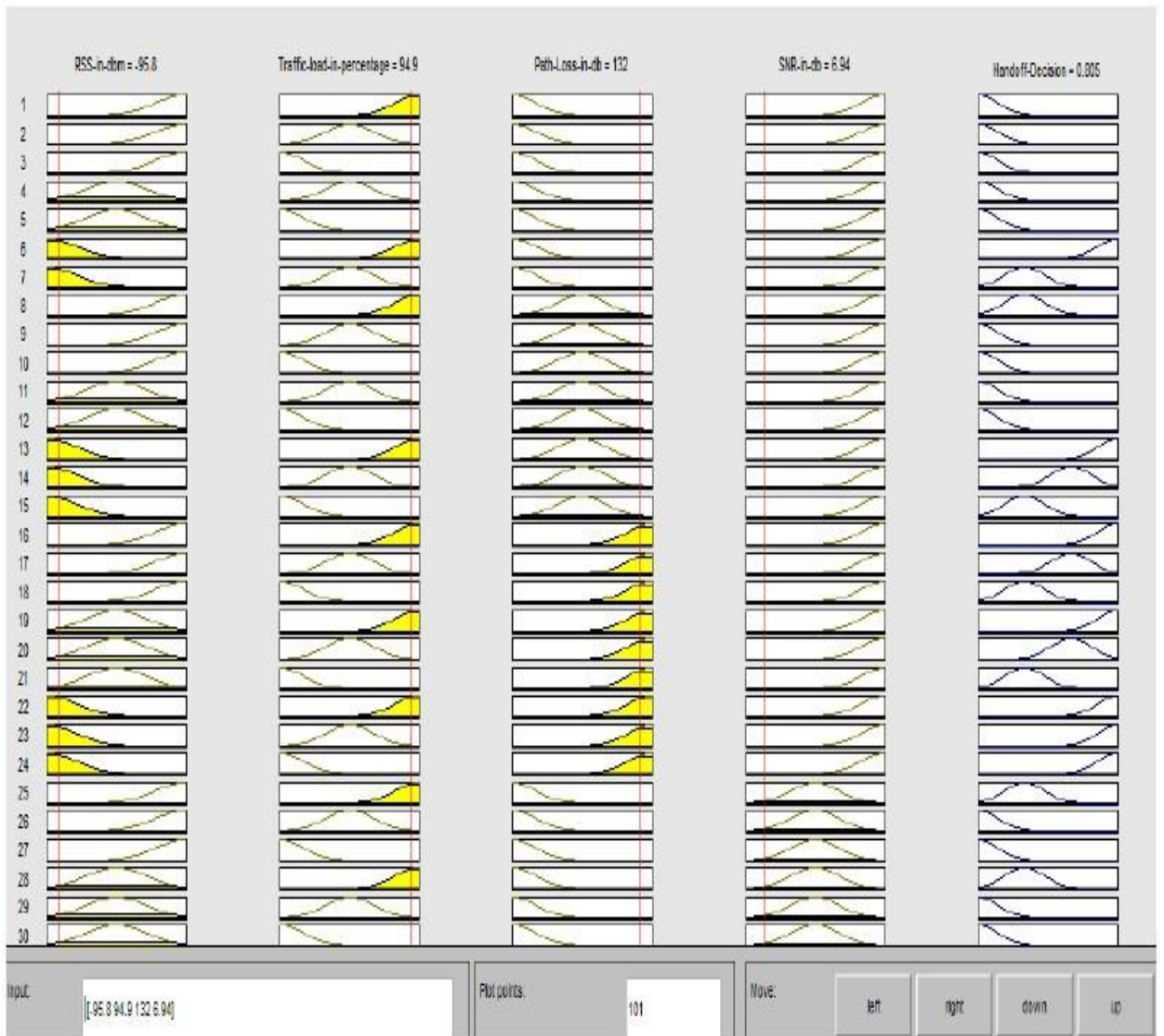
Figure 4. 18: Rule Base evaluations when all the four parameters are worst [45] The rule base evaluations when the four parameters were worst are shown in Figure 4.18 that was developed by authors in [45]. The output of the system for this case was 0.805.
