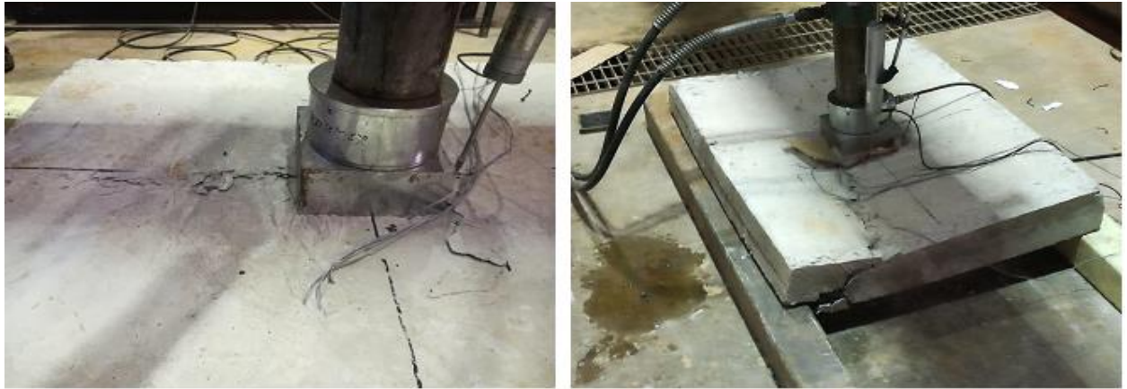
Plate 4-7 Progressive failure of the deck slab with longitudinal cracks increasing in size till failure.
