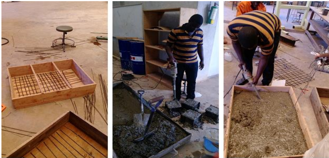
Plate 3-5 Fabrication process of the Deck Slab model in the laboratory
