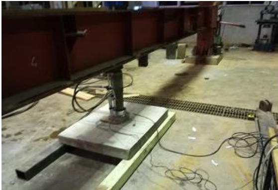
Plate 3-7 Strain gauges connected to the transducer and the LVDT connected to the Loading Cell to measure deflection at the centre of the slab.
