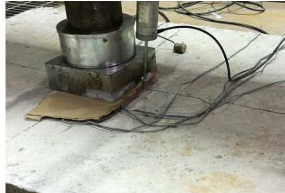
Plate 3-7 Strain gauges connected to the transducer and the LVDT connected to the Loading Cell to measure deflection at the centre of the slab.
