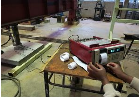
Plate 3-6 Transducer being configured prior to testing and Loading using a Load cell.
