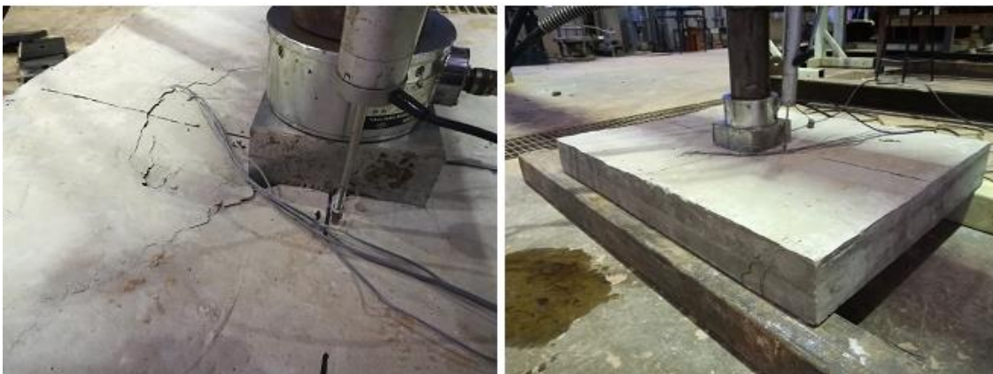
Plate 4-9 Progressive failure of the deck during the testing with punching shear observed
