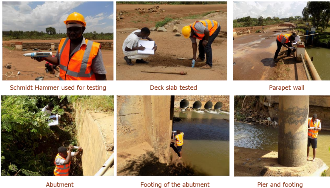
Plate 3-1 Schmidt Rebound Hammer used for the in-situ testing of the compressive strength
