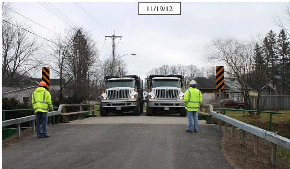
Plate 2-1 Traffic load tests to determine load capacity of composite decking
