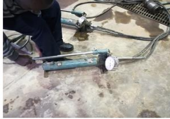
Plate 3-6 Transducer being configured prior to testing and Loading using a Load cell.
