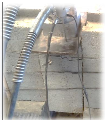
Plate 4.7: Failure mode for R-DHSBs specimen
