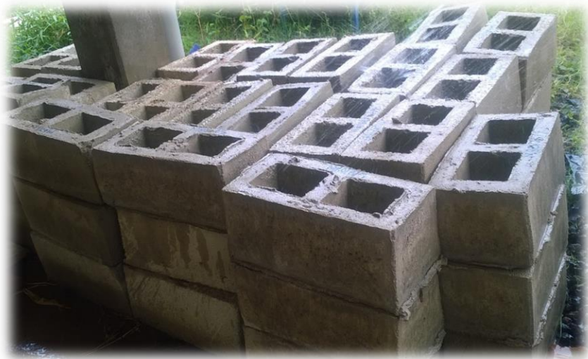
D2: Sandcrete blocks containing Lateritic sand: Marine sand blend stacked for curing
