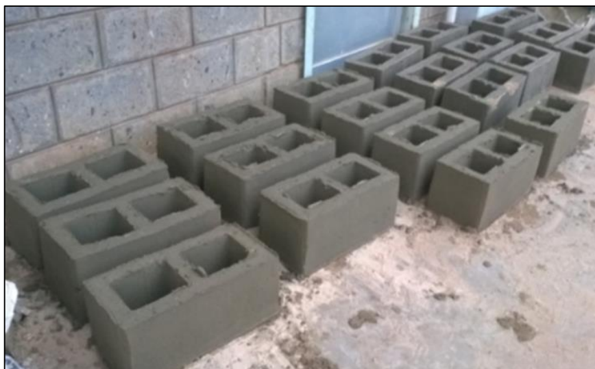
Plate 3.1: Sandcrete blocks made by blending clean lateritic and marine sand
