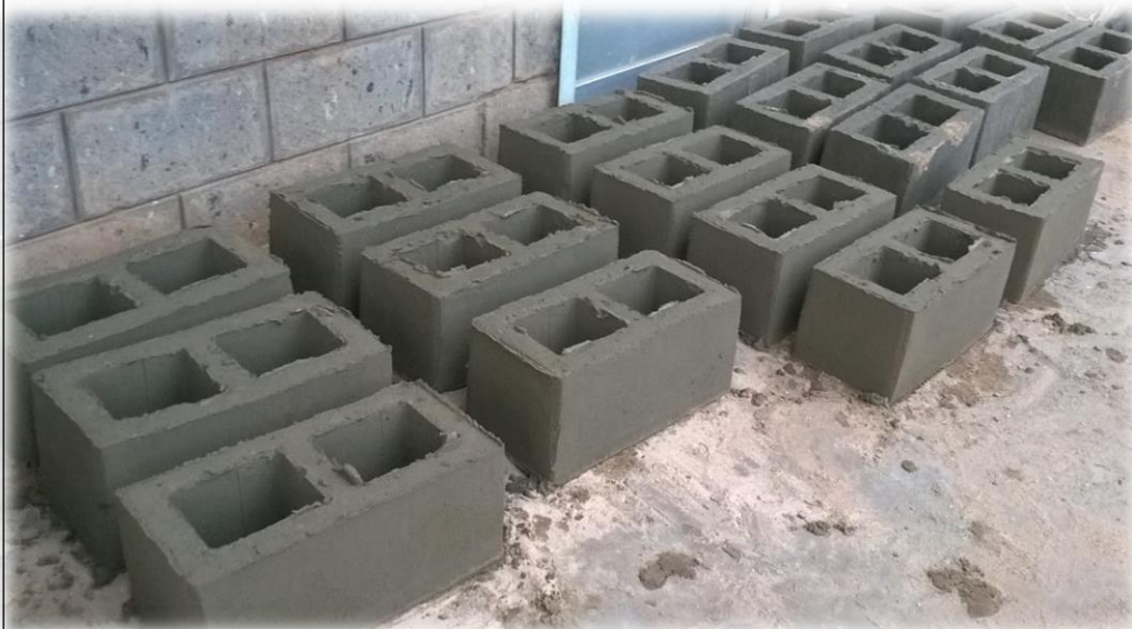
D4: Sandcrete blocks immediately after casting
