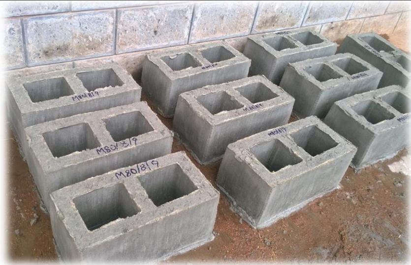
D1: Sandcrete blocks containing 20:80 Lateritic sand: Marine sand blend.
