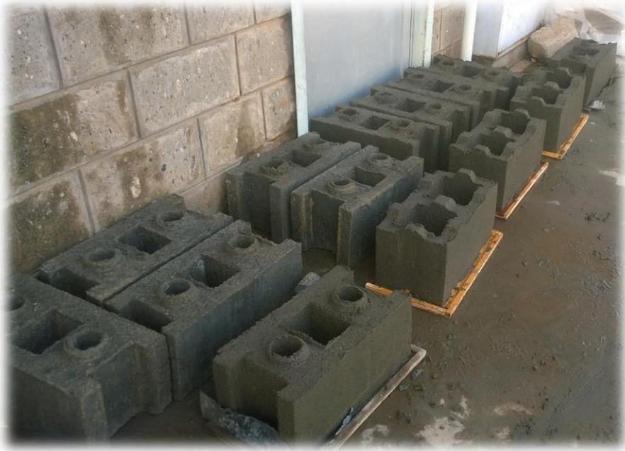
D5: Dry stack hollow sandcrete blocks
