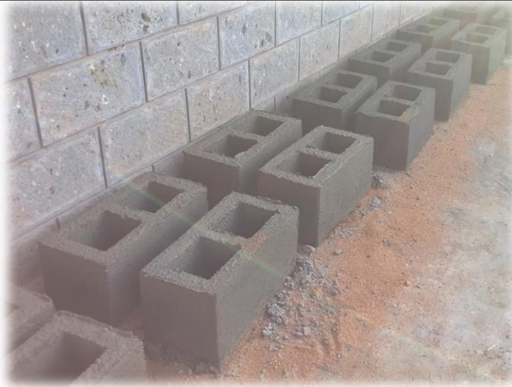
D3: Sandcrete blocks containing SBA at varying content.
