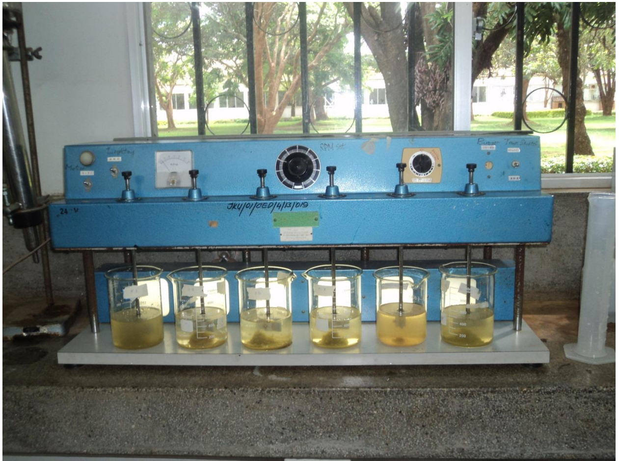
Figure B.3: Jar test for Opuntia Spp. bio-coagulant in River water treatment
