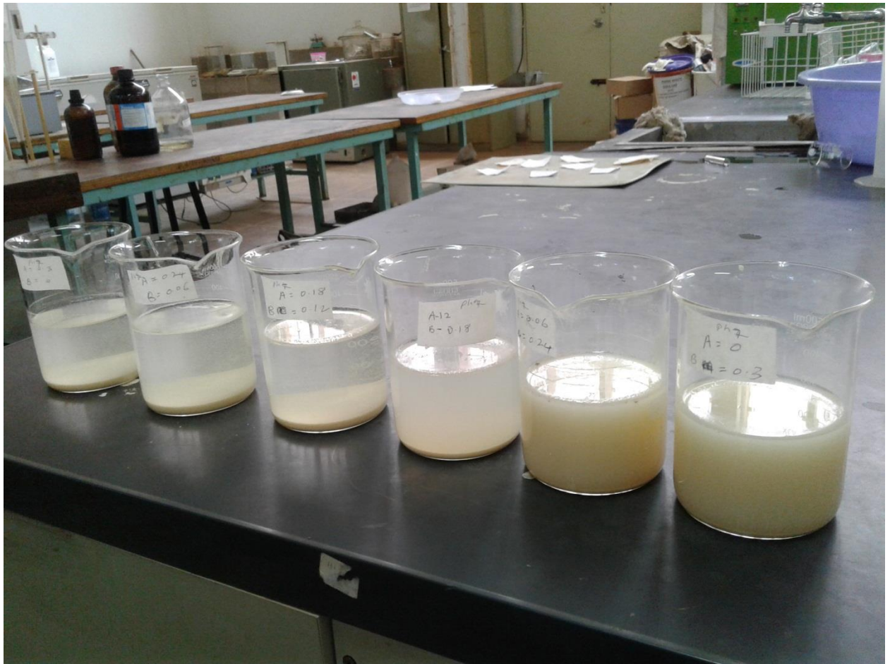
Figure B.5: Jar test for alum and Banana pith coagulants in industrial (paint) wastewater treatment
