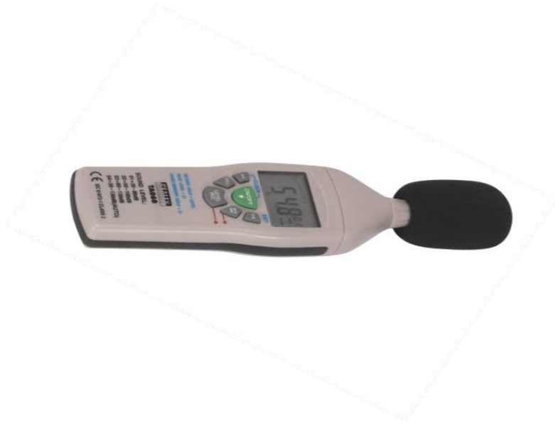
Figure 3.2: Meter used to measure noise levels
