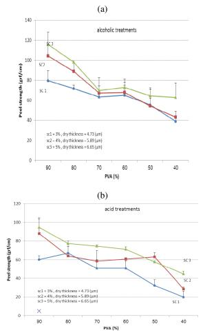
**Figure 2**. The effect of solid content on peel strength of paper in different (a) alcoholic treatments, (b) acid treatments.
