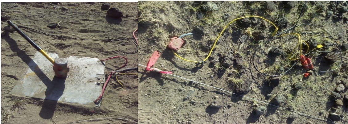
Figure 2. 2: Steel alloy plate fitted with a trigger and a sledge hammer (left), geophones placed firmly in the ground a long a line, also seen is a rope calibrated with a red tape; the position at which the geophone is placed, (right).
