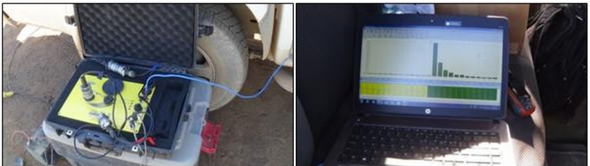
Figure 2. 1: DAQLink III and Laptop for data collection
