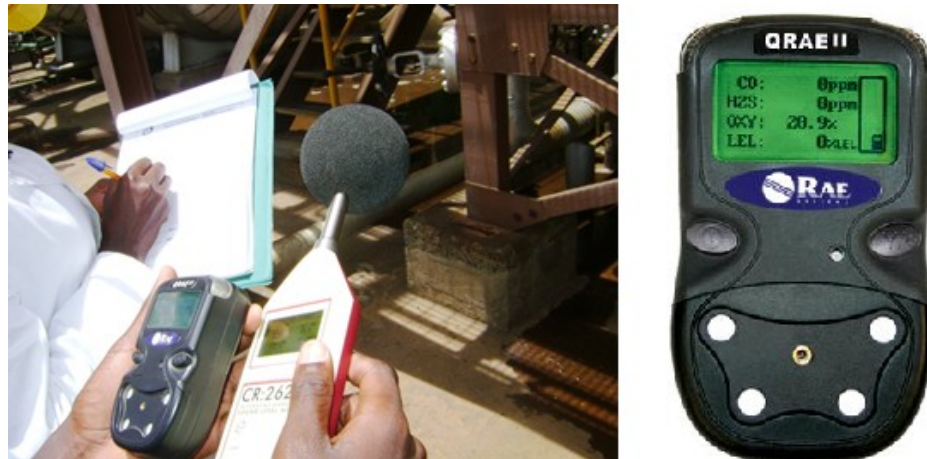
Plate 3.1: Measuring H 2 S at the cooling tower in Olkaria II using QRAEII 4 gas monitor
