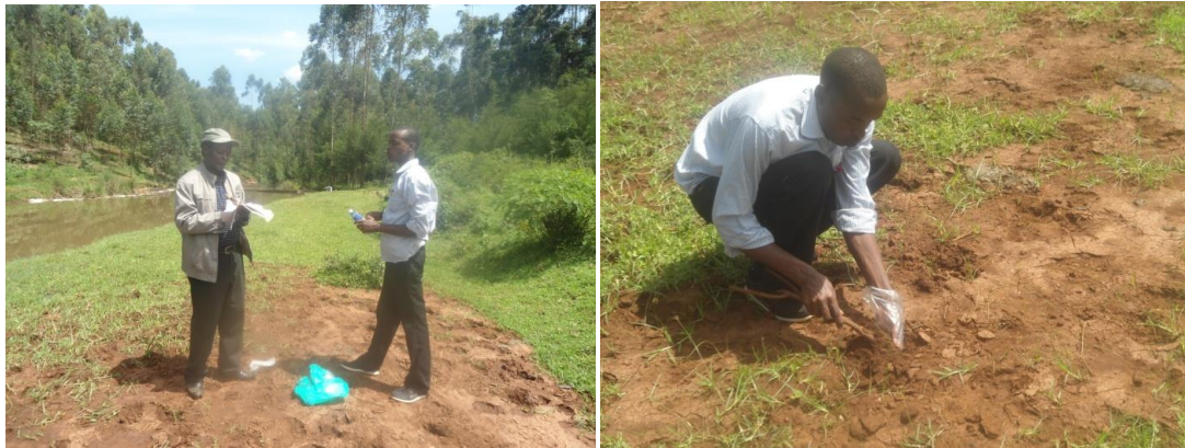
Figure3.4: Shows sampling of soil sediments trapped by Kikuyu Grass along the river bank.
