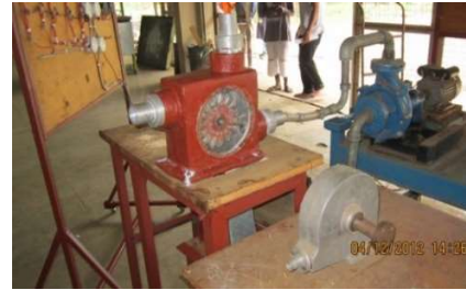
Pelton wheel turbine for micro-hydro power generation
