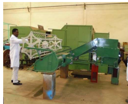
Rice combine harvester developed at JKUAT
