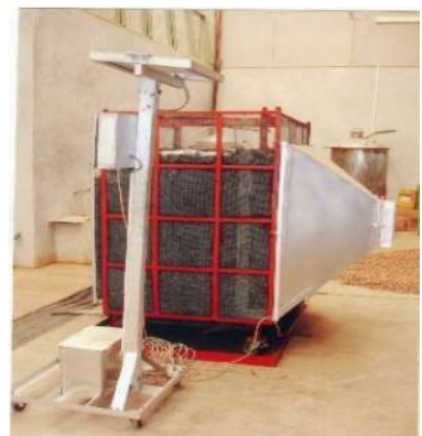
A charcoal cooler for extending shelf life for mangoes
