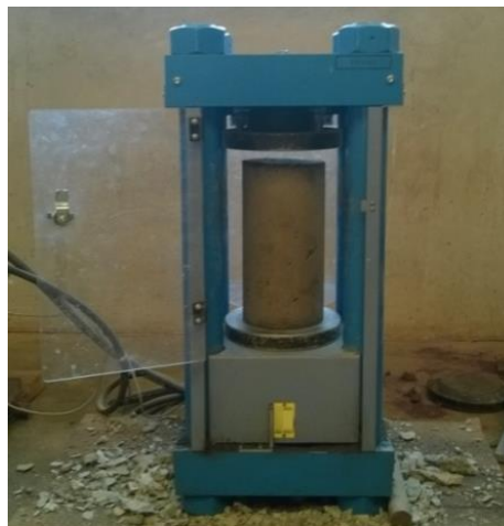
Plate 3.3: Compressive strength testing
