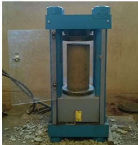
Fig. 8. Compressive strength testing
