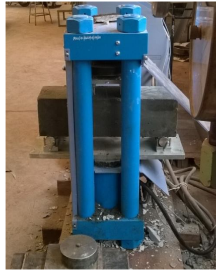
Fig. 9. Flexural strength testing
