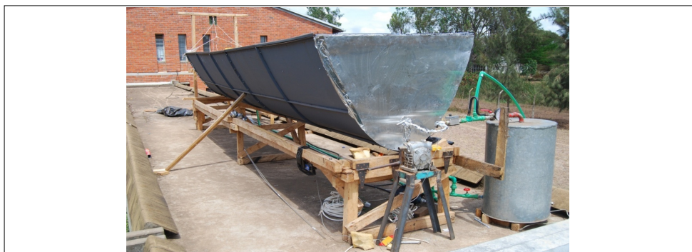
Figure 1: Fabricated prototype parabolic trough solar concentrator for steam production
